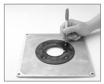
Figure 12. Marking insert for drilling.
